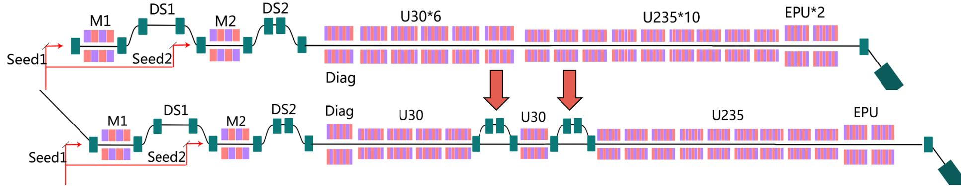
➤ EEHG-HGHG @ 3nm (1.4 GeV, U30, Gap: 16.9 mm, K=1; U235, Gap: 9.4 mm, K=1.33)
