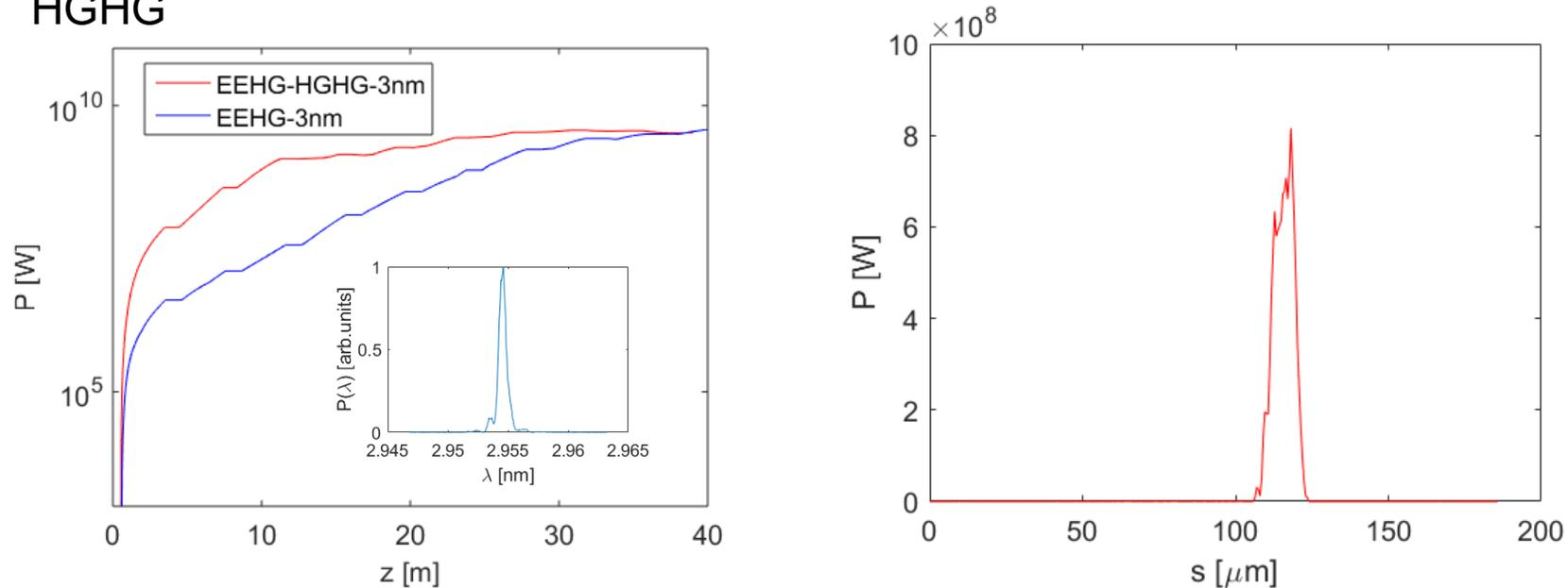
Lower energy spread and higher bunching significantly reduce the gain length at 3 nm
