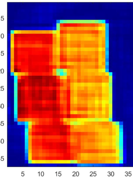
Beam shape on SiN:  $\sim 10\mu\text{m}$
