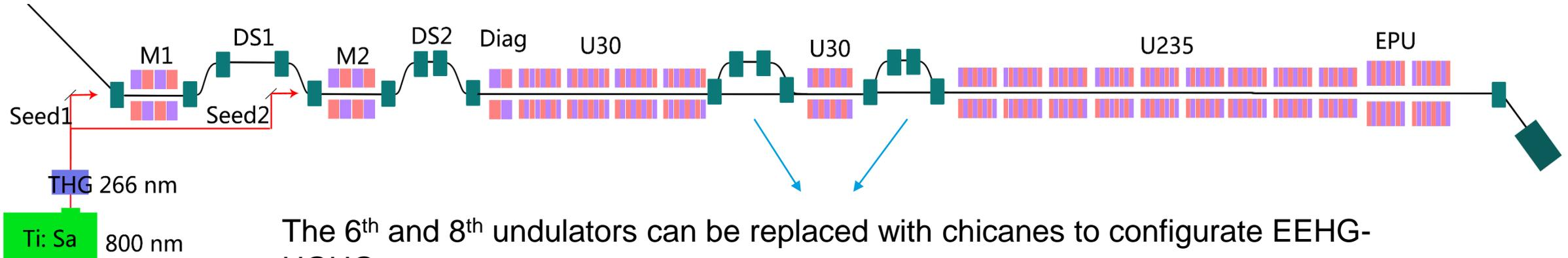
The 6<sup>th</sup> and 8<sup>th</sup> undulators can be replaced with chicanes to configurate EEHG-HGHG
