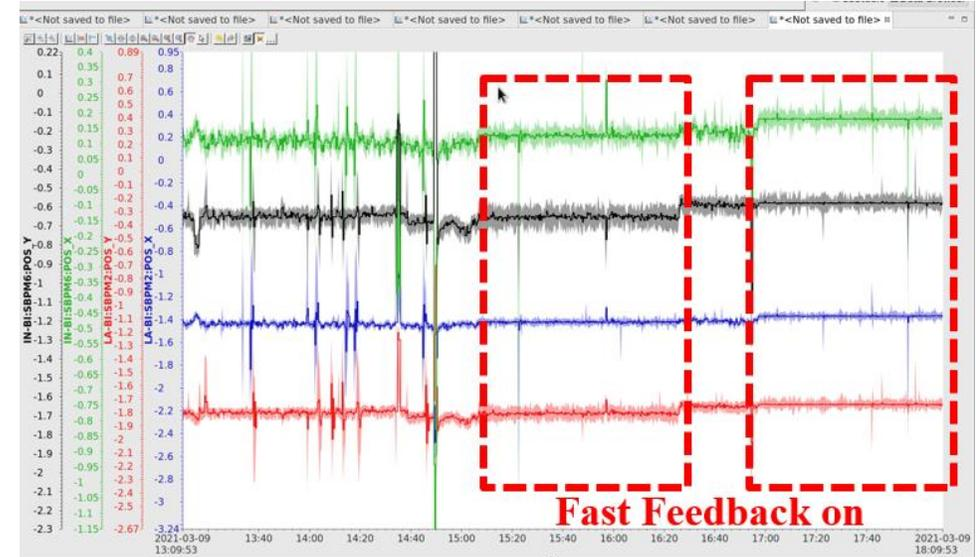
Beam trajectory and jitter along the whole machine, jitter: 10-20  $\mu\text{m}$  (rms)
