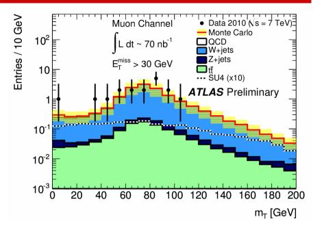
Required 1 lepton with  $p_T > 20 \text{ GeV}$  and 2 jets with  $p_T > 30 \text{ GeV}$  and MET > 30 GeV
