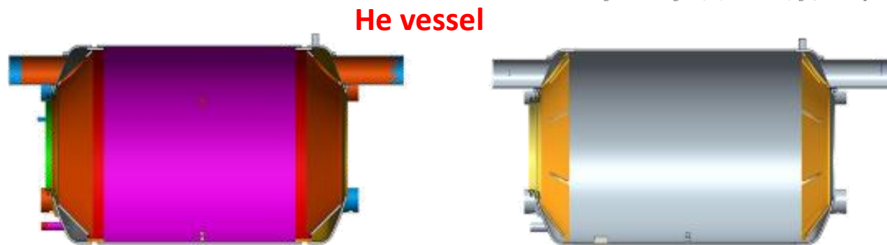
Figure 3.16. Original (left) versus new (right) vacuum jacket design.
