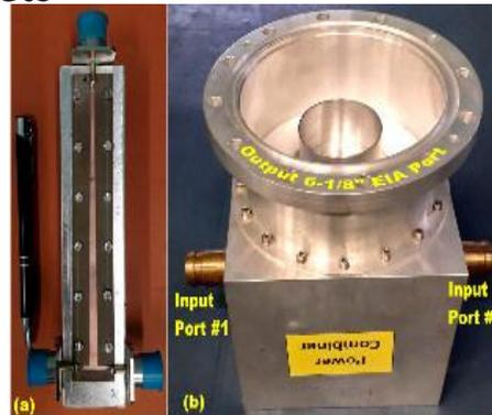
Fabricated 2-port (a) tapered microstrip divider (b) High power combiner with 6-1/8" input and output ports.
