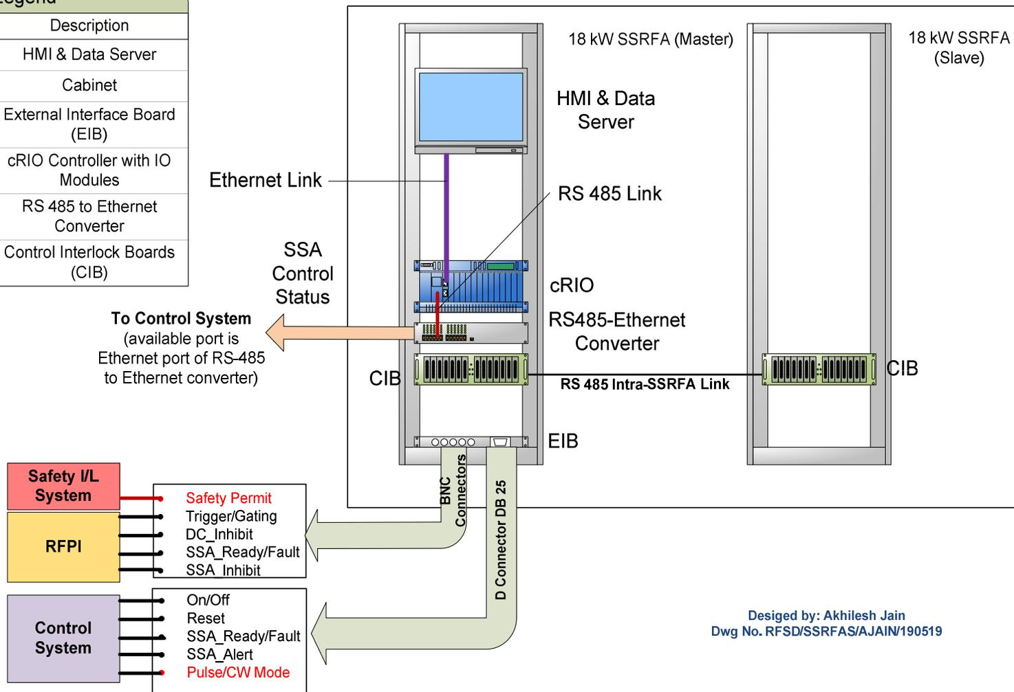
Low power amplifier and control/interlock hardware is different in both units, all other details are same for both master and slave units.
