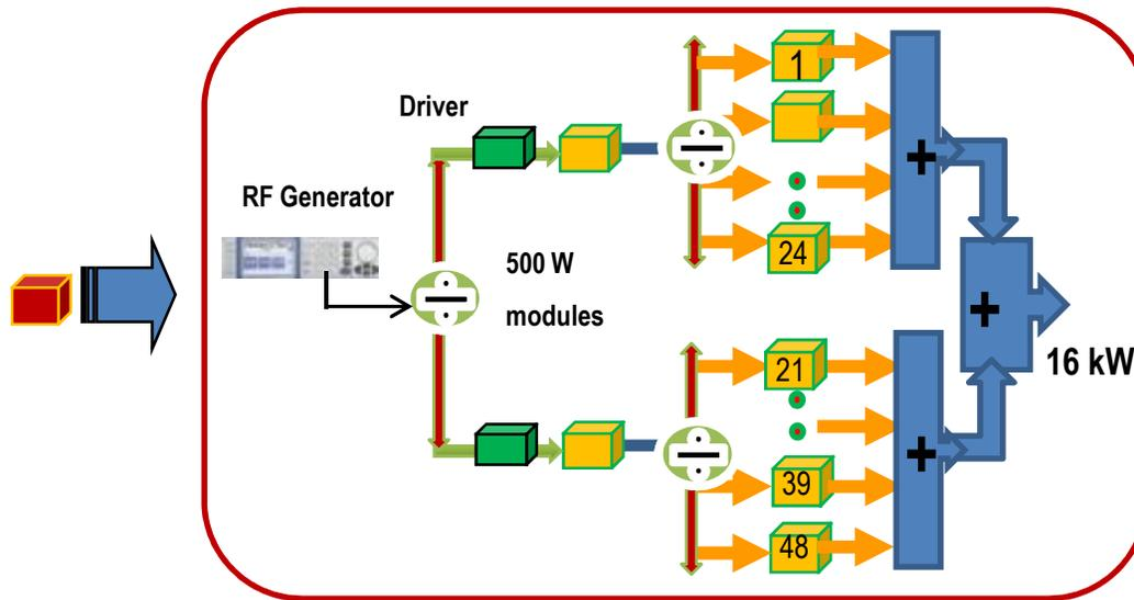
16 kW Unit scheme used in 32kW Amplifier
