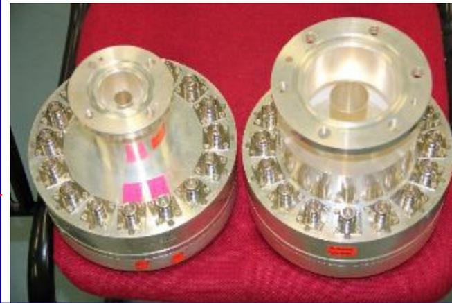
48 way Power Divider (left) and Combiner (20 kW power handling)
