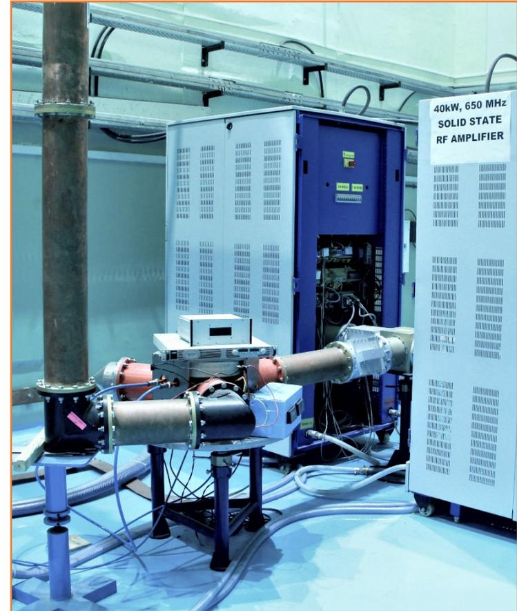
High power test set up for testing superconducting RF cavities
