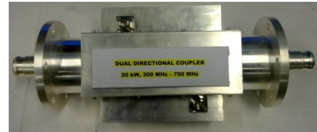
Designed 1 kW, 5 kW and 20 kW directional couplers
