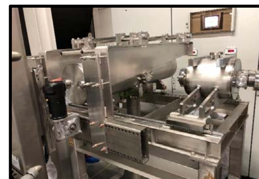
Cavity lowered onto support frame and aligned with solenoid
