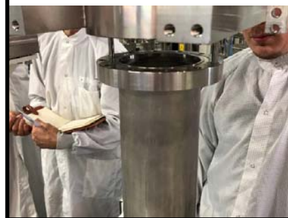
Cavity-coupler alignment and assembly
