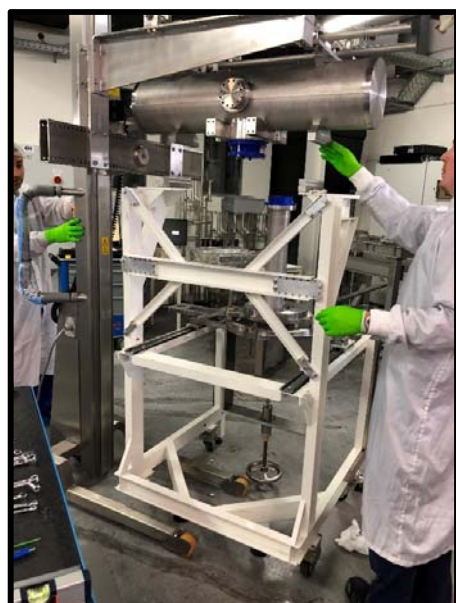
Cavity lowered on cavity-coupler assembly frame
