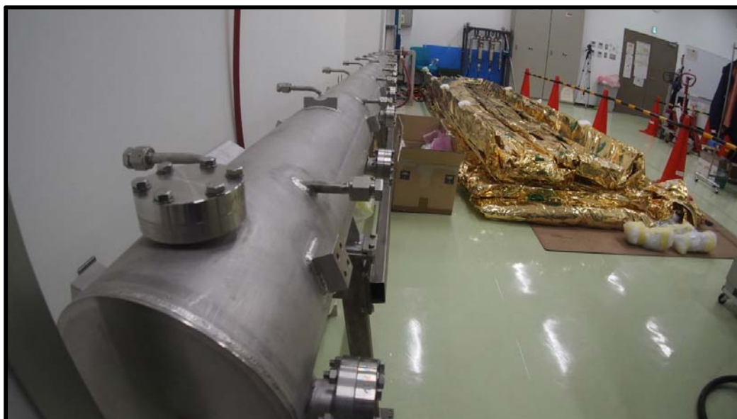
Phase separator + magnetic shield
