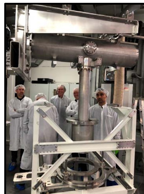
Transfer of cavity- coupler to cold mass support frame
