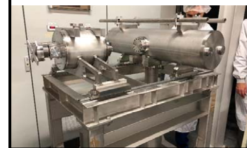
Cavity lowered onto support frame and aligned with solenoid
