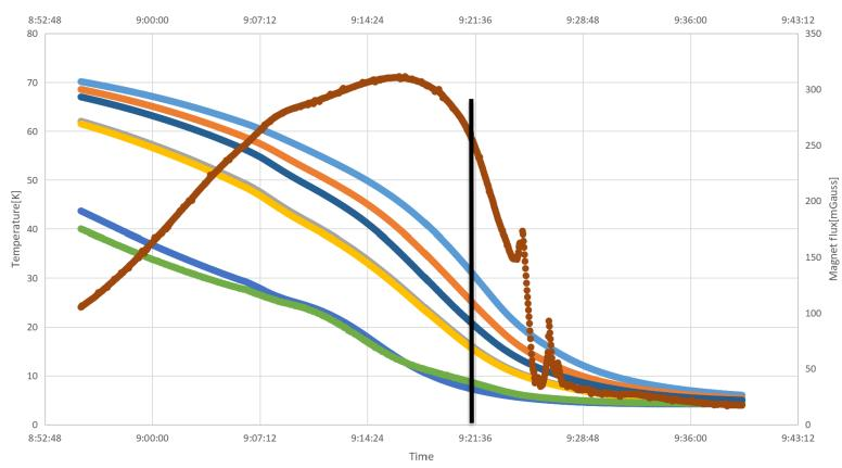
Nb Copper HWR010 cavity First Cool down 40-6K
