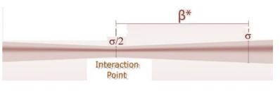
\*\*Sometimes  $\beta$  is referred as the distance from the focus point that the beam width is twice as wide as the focus point.\*\*
