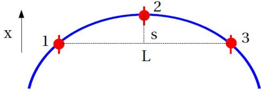
Error propagation:  $\sigma_s^2 = \sigma_2^2 + \sigma_1^2/4 + \sigma_3^2/4$  (usually Gaussian)
