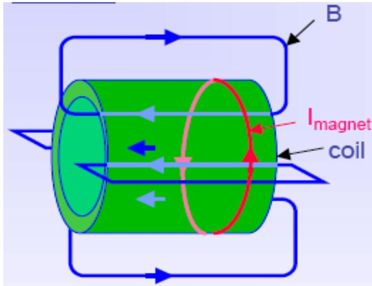
Field direction along beam axis.
