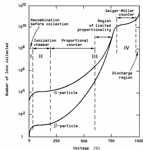
Number of electron-ion pairs of a charged particle traversing a gas detector vs the voltage applied
