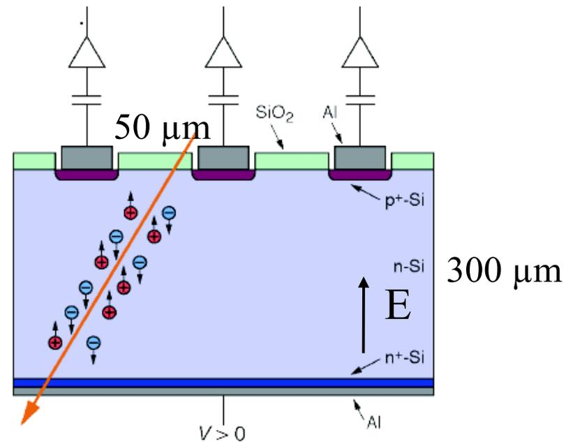
Figure 2.8: Schematic structure of a CMS silicon microstrip sensor.
