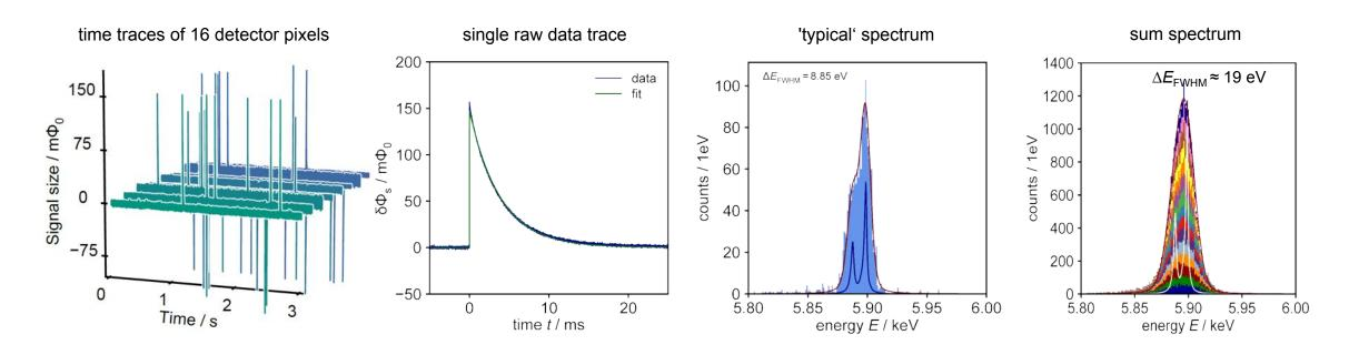
first truely multiplexing demonstration of magnetic microcalorimeters some issues still to be resolved (ongoing)
