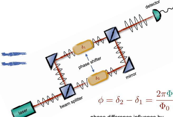
phase difference influence by magnetic flux threading SQUID loop
