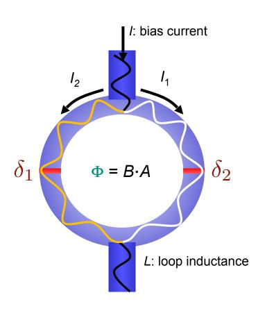
SQUID = quantum electromagnetic equivalent of an optical interferometer
