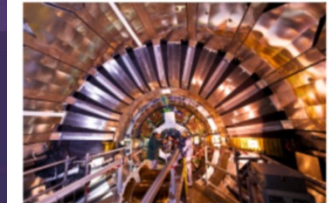
Installation of the CMS Central Tracking Detector with 10 million read-out channels and using silicon detectors covering an area of over 200 m 2 . (© CERN)
