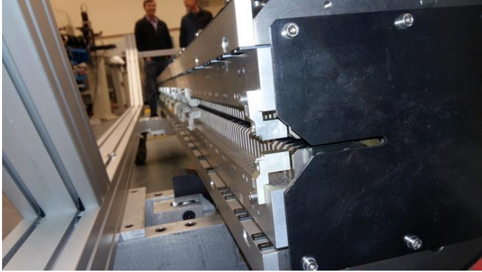
Some Properties of the LCLS-I undulator
