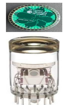
*The Wavelength-Shifting Optical Module (Sensors 2022, 22, 1385)*
