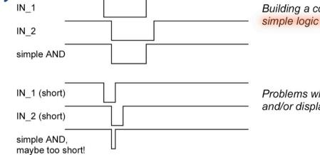
Building a coincidence by simple logic AND function.
