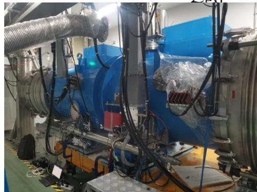
Fig. Eight-cavity and Single-cavity cryomodules
