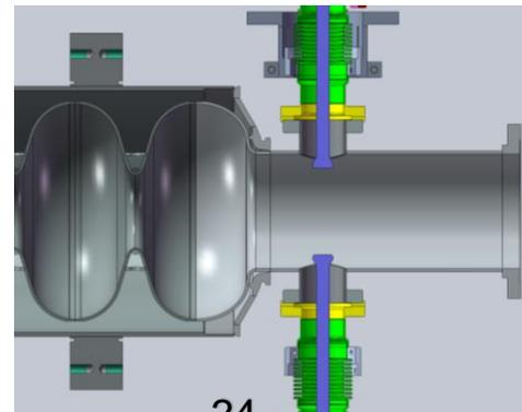
Fig. FPC for double-fed cavity
