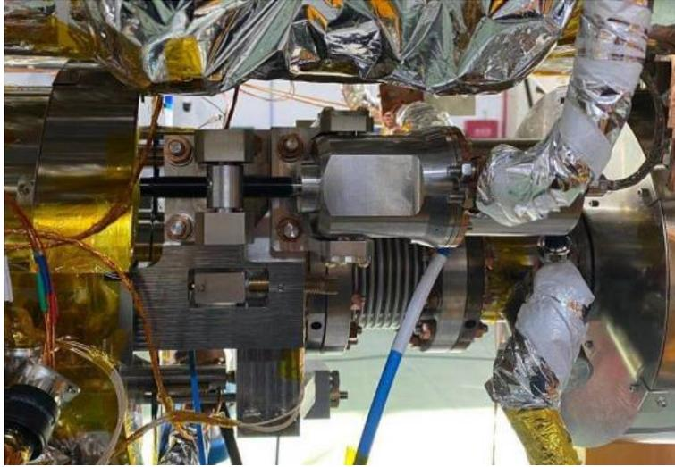
Tuner mounted on cavity
