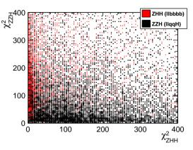
• With ErrorFlow  $\rightarrow$  larger separation of signal (*ZHH*) and background (*ZZH*)
