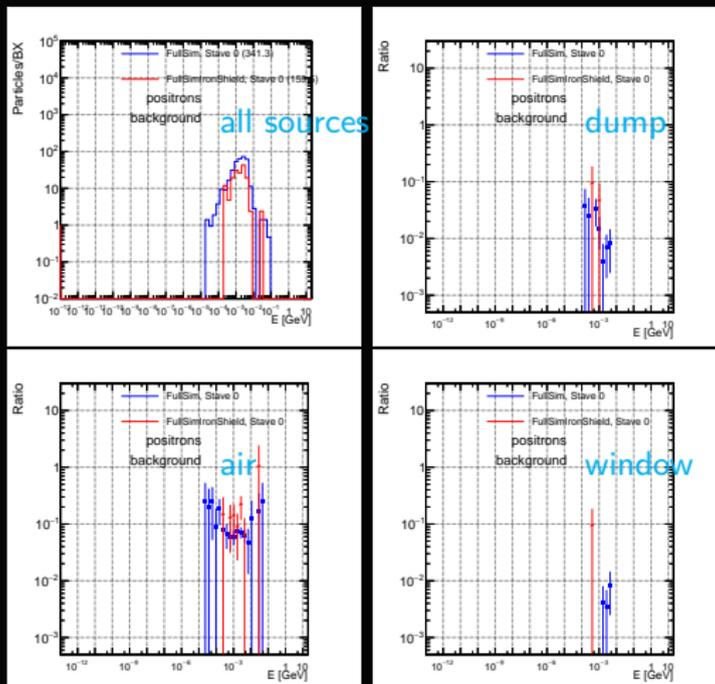
53% less positron with neutron absorber and iron shield.
