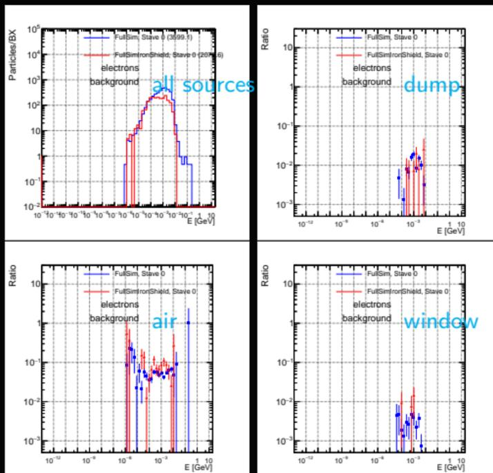
42% less electron with neutron absorber and iron shield.
