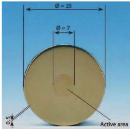
Geometry -> alpha are emitted in a cone with semi-aperture 28.3 deg.
