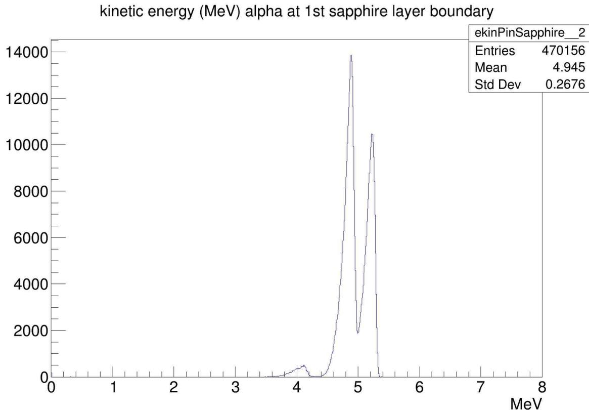
The average energy loss of alpha particles in the 6.5 mm air + 100 nm metallization is
