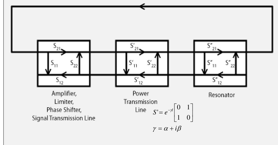
Condition for self-excited oscillation:  $\left(S_{21}S''_{21} + S_{22}S''_{11}e^{-\gamma t}\right)e^{-\gamma t} = 1$
