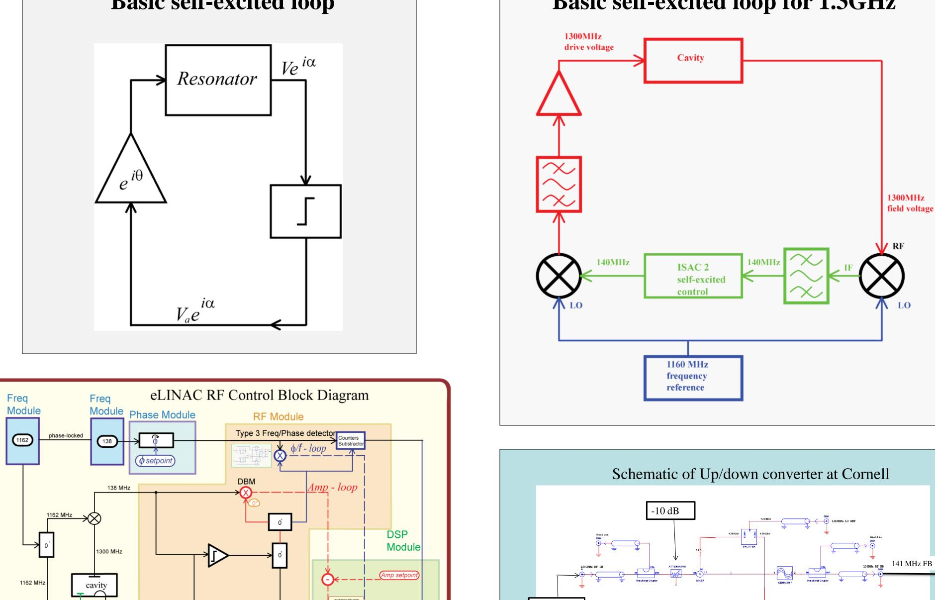
Using a fixed LO frequency of 1160MHz and varying the loop phase alone, we have been able to lock to 3 different cavity modes.
