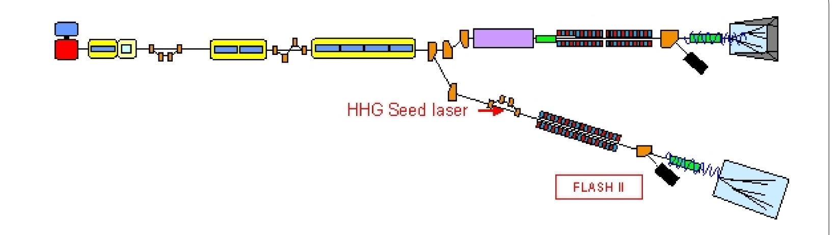
The electron gun is on the left, the experimental hall on the right. Behind the last accelerating module, the beam is switched between FLASH I, which is the present undulator line, and FLASH II, which is the upgrade.
