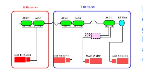
Established the possibility of operating the cavities with two gradient levels (pulse to pulse and intra pulse) so that they can be run at a high gradient along with (during) SASE operation.
