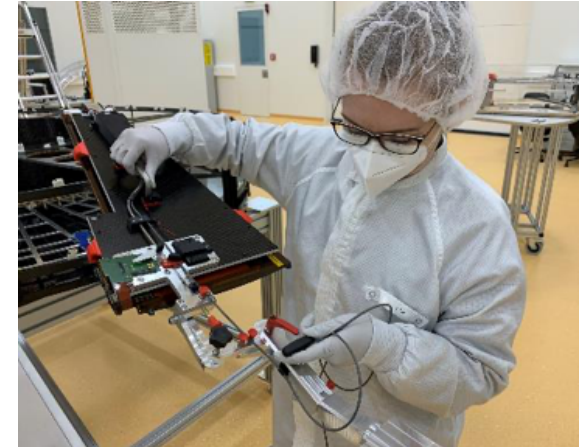
Petal insertion procedure tested with end-cap mock-up
