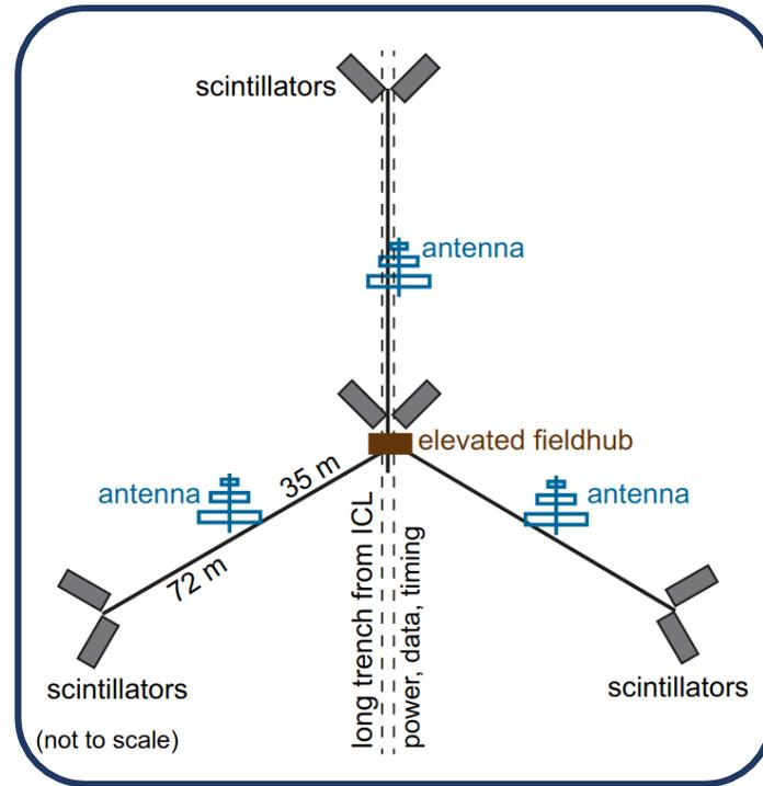
4 pairs of scintillation detectors + 3 antennas
