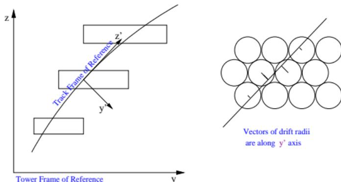
A MILLEPEDE-like algorithm was written for alignment of a sector of the ATLAS Muon Detector using straight muon tracks
