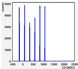
Pixel address in 5 data: C1,C0 d-columns 0..25 A2, A1, A0 rows 0..159 each with 6 analog levels (2.5 bit). All well separated.
