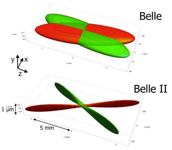
Dimensions of luminous region at Belle II are 10/0.2/250 µm (x/y/z) compared to 100/1/6'000 µm at Belle. Ultimately, *y* size expected to be decreased to ~60 nm
