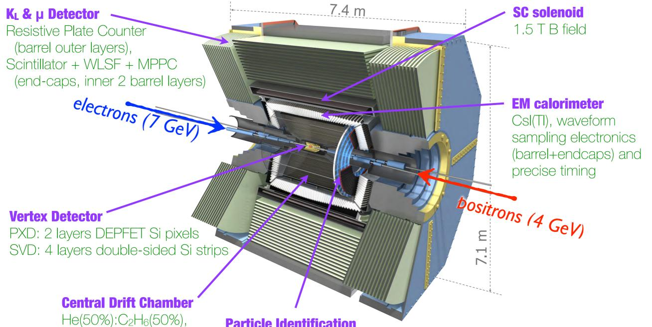
small cells, long lever arm, fast electronics
