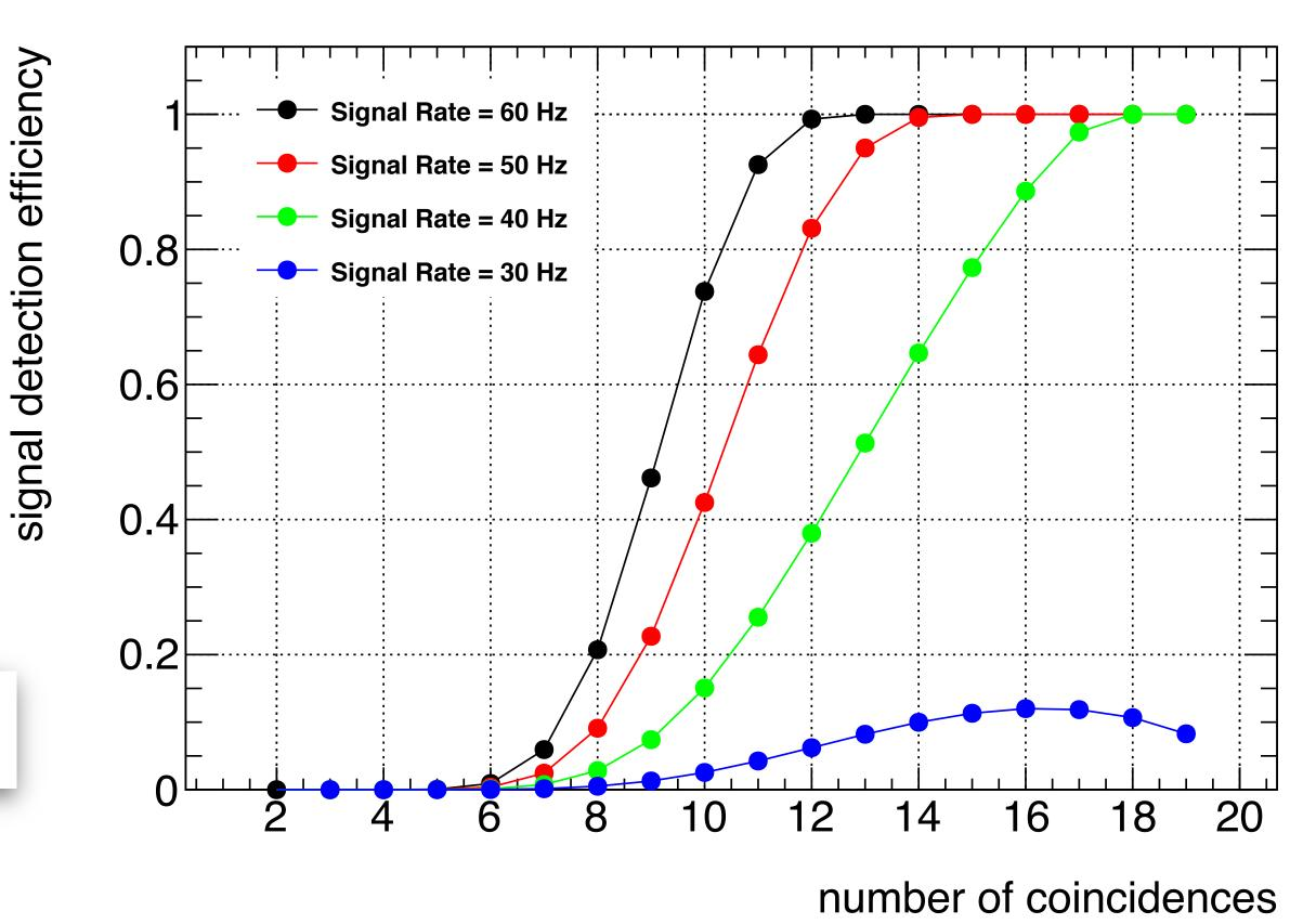
With 20 detectors a photon flux of 40 Hz can be detected with an efficiency of 1 within a coincidence interval of 32ms
