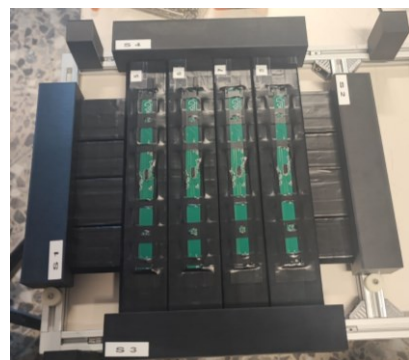
PSD prototypes under tests during BT campaigns at CERN and CNAO (2022-2023...)
