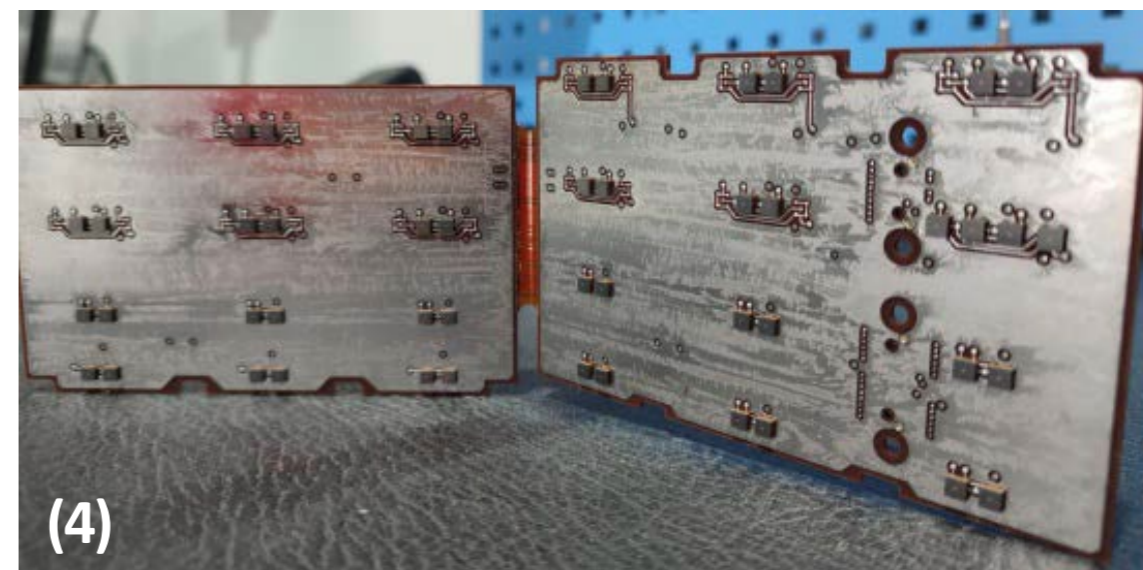
(4) The Rigid-Flex PCB readout hosting the SiPMs of the Plastic Scintillator Tower (PST)
