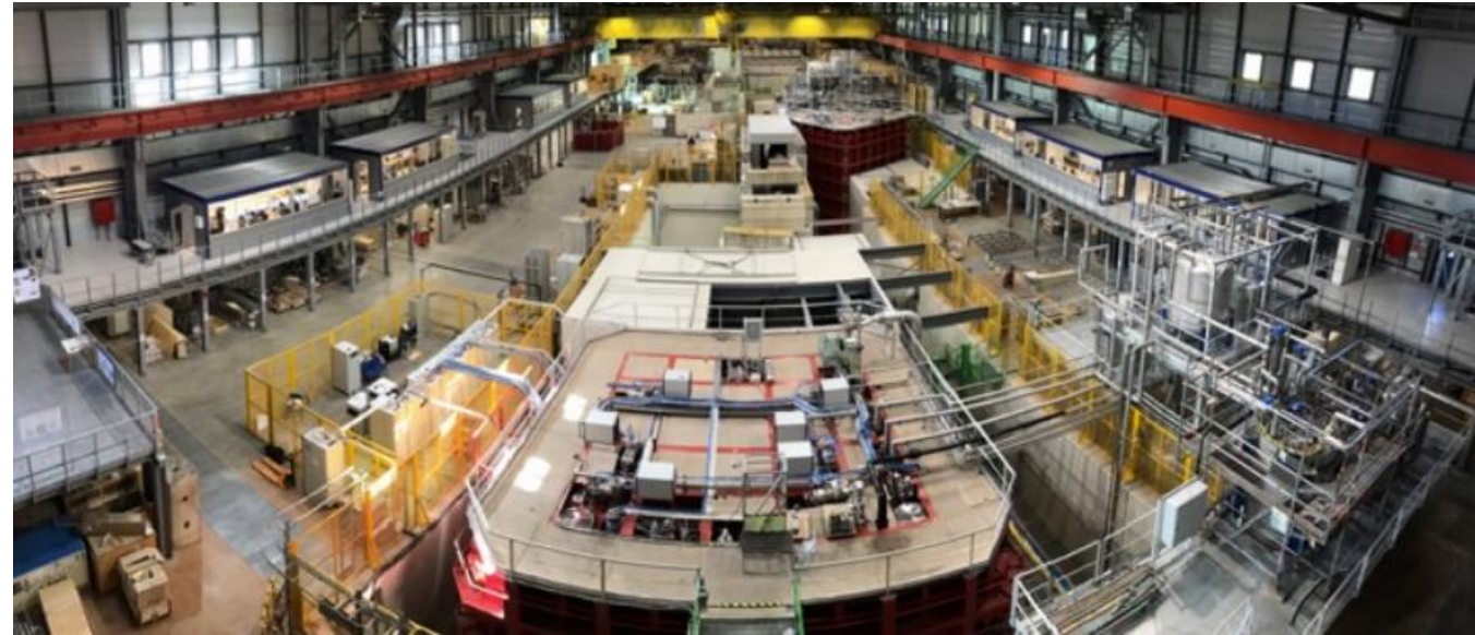
Panoramic view of the CERN Neutrino Platform with ProtoDUNE-SP cryostat (bottom). Beam travels from top to bottom.
