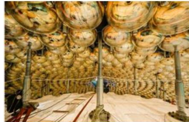
PMT installed in detector
