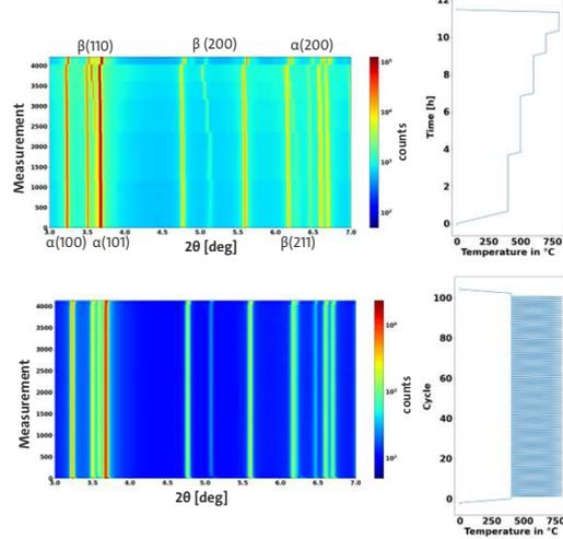
Reference measurement with continuous heating
