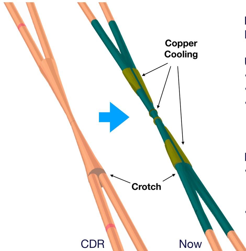
**Engineered CAD model** of AlBeMet162 beam pipe developed by INFN-LNF (many thanks to F. Franesini) imported in **Key4hep**.
