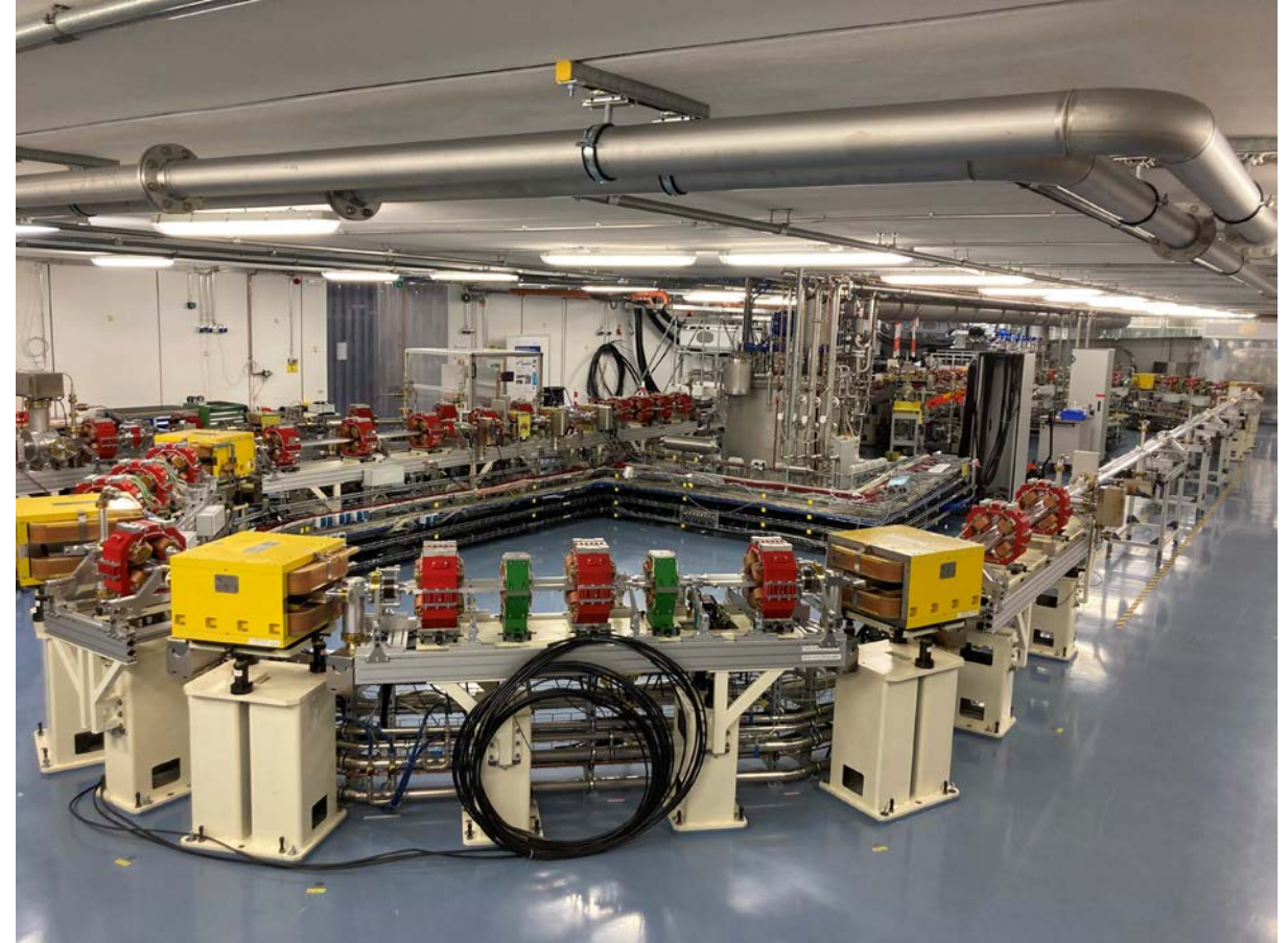
Vacuum system complete, realigned with coordinate system adjusted to building (moved over the years) Cabling of diagnostics well advanced
