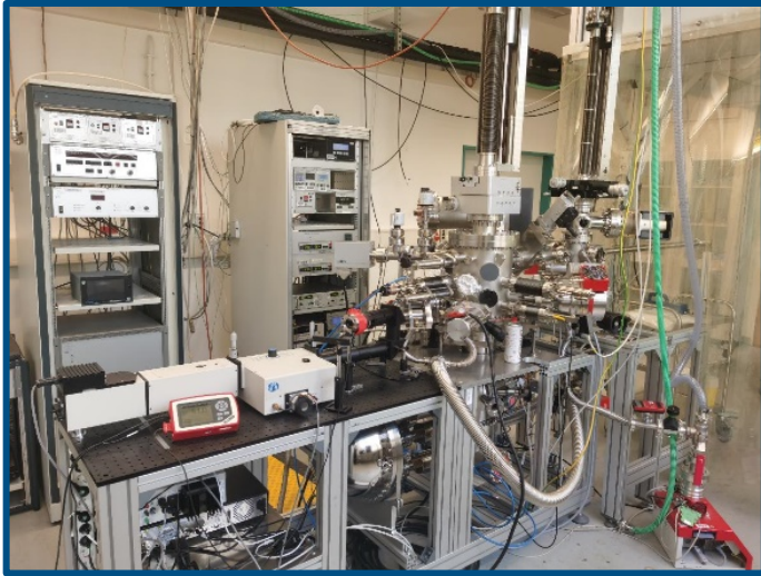
Photocathode Preparation & Analysis System
