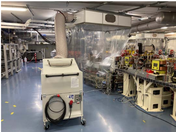
Rail system at ceiling to allow ISO5 flow-boxes everywhere at the machine to avoid particulates
