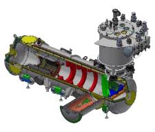
Large bore (Ø = 760 mm) cryostat allows operation of all prototypes Fits into the 1600 mm warm bore of MORPURGO magnet at CERN
