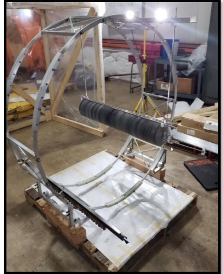
The segmented geometry helps to reduce electron energy losses (improving momentum resolution)
