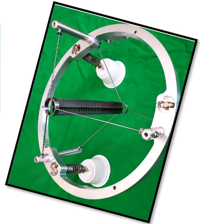
**The production target with its support structure**
