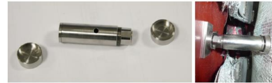
Figure 10: Outer pressure prop parts (left) and prop inserted into the cryostat (right).
