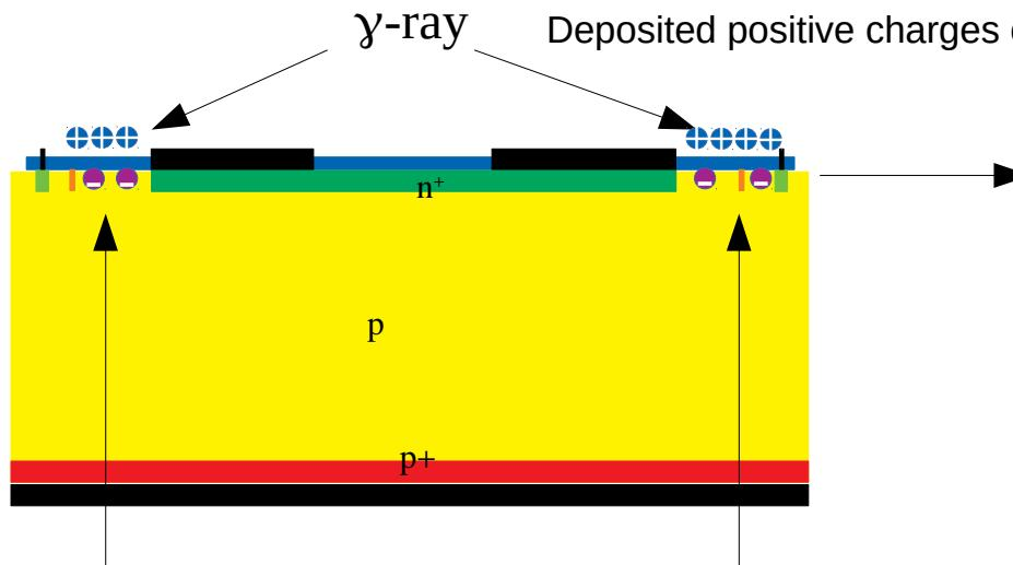
As the accumulation of positive charges on the  $\text{SiO}_2$ , The resistivity between guard-ring and pad are changed.
