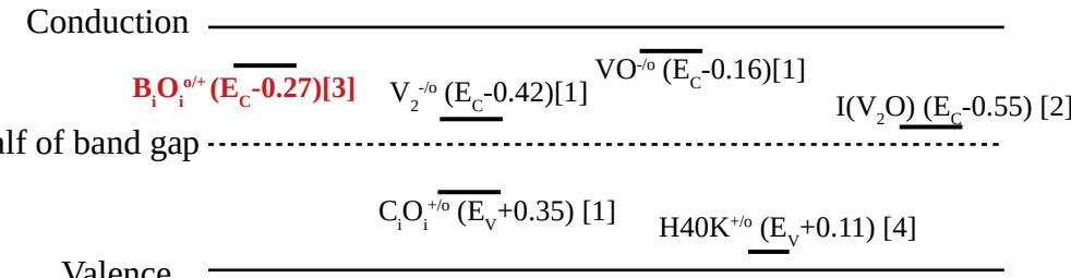
**“The radiation damage induced defect in p-type silicon,  $\text{BiO}_i$  is investigated”**
