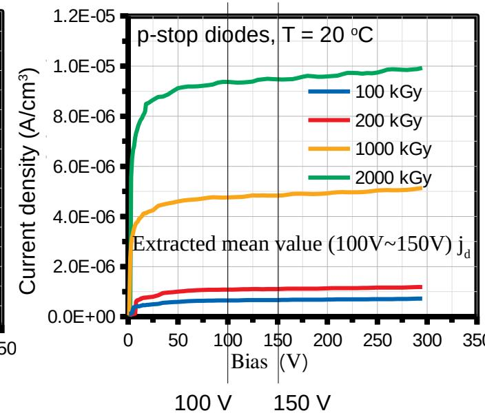
Current density given by I-V and C-V (100 kHz for p-stop diodes)
