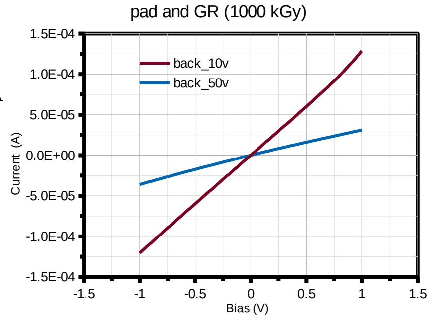
The definition of conductance( $\sigma$ ):  $\sigma = dI/dV$
