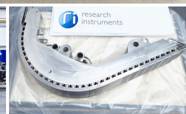
IVT 20 MW/m 2 @2000C W monoblocks brazed to CuCrZr-pipe
