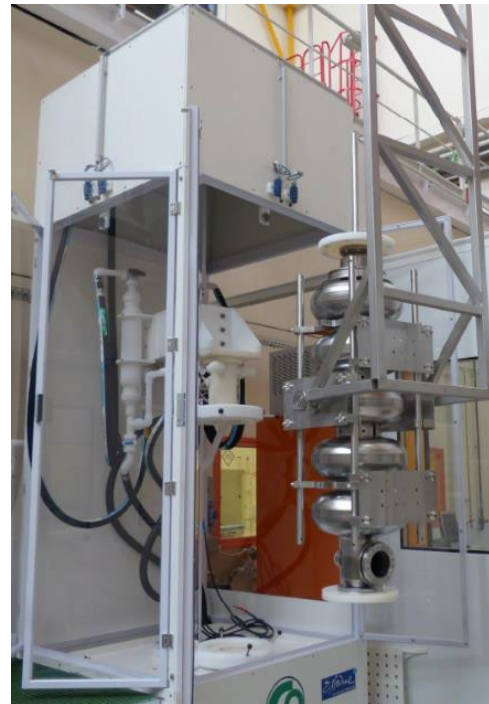
Vertical electropolishing cabinet
