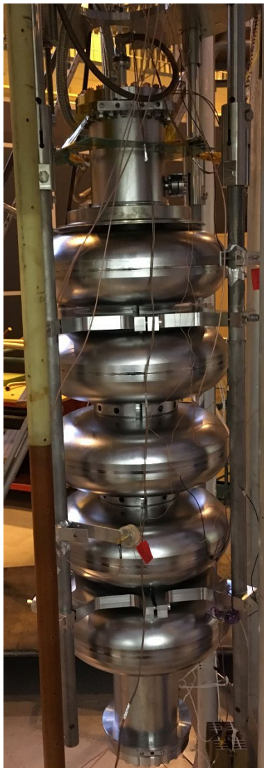
ESS High beta cavity installed in VT stand
