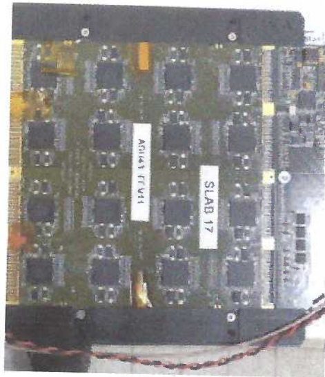
Figure 19: A fully instrumented sensor plane for ECAL-E. The SKIROC2 ASICs are positioned of the silicon pad sensor
