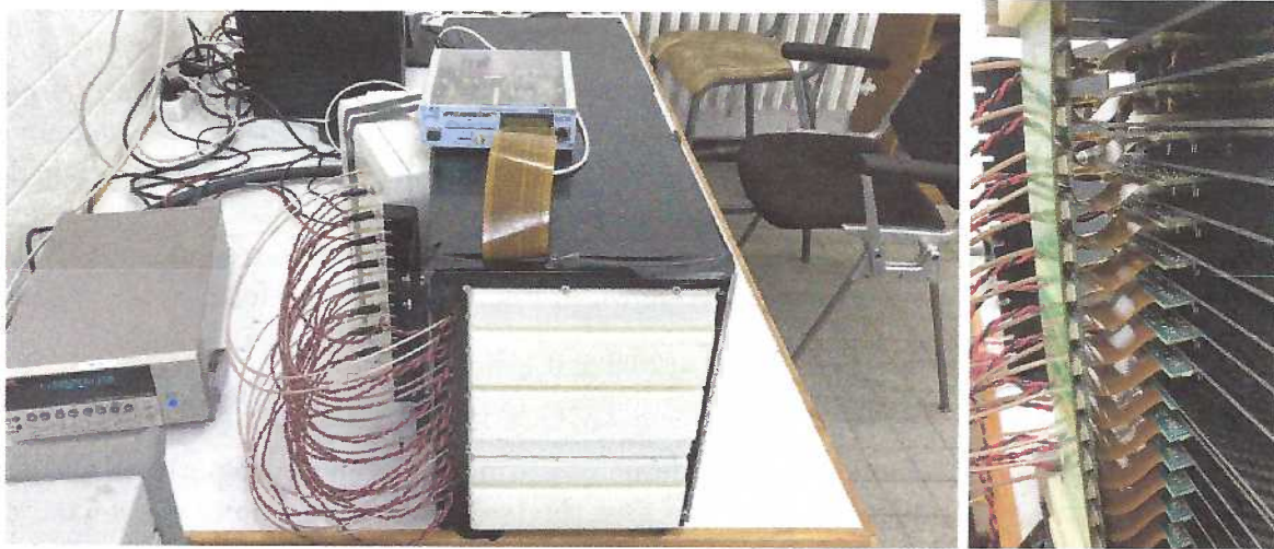
Figure 6: Left: picture of the 15 layer stack of ECAL-E. Visible are the mechanical housing the HV and LV cabling and the flat Kapton cable for the readout of the 15360 pads of the stack. Right: Zoom into the extremities of the stack to appreciate the compactness of the ensemble.
