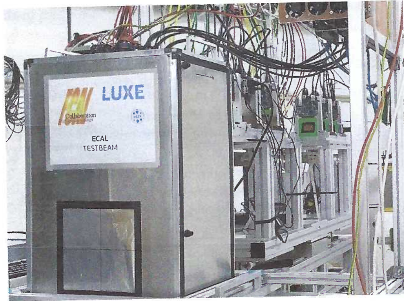
Figure 23: The test-beam set-up for the measurements of the sensor response. Left in the foreground is the detector box with the sensors and FE-electronics inside. In the background right the pixel telescope is shown , used to measure the electron trajectory.
