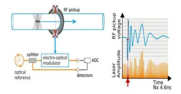
Here updating the efforts made toward creating a BAM that uses rod-shaped pickups installed on a printed circuit board and ultra-wideband travelling-wave electro-optic modulators with low operating voltages.
