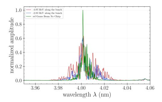
Effect of Chirp on wavelength, bandwidth and Power of
