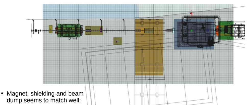
• Shielding is wider in X direction in 3D CAD.
