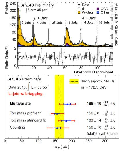
$$\sigma_{t\bar{t}} = 186 \pm 10(\text{stat.})^{+21}_{-20}(\text{syst.}) \pm 6(\text{lumi.}) \text{ pb}$$
