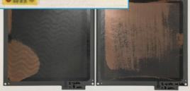
Flaking due to high stress at low temperature
