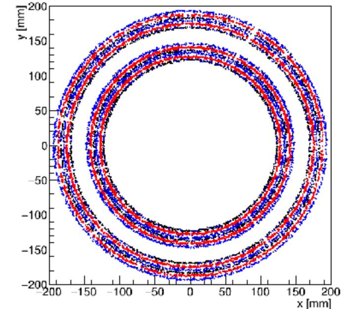
Hits reconstructed in the **middle** of the gas gap using **entry** and **exit** position of the tracks
