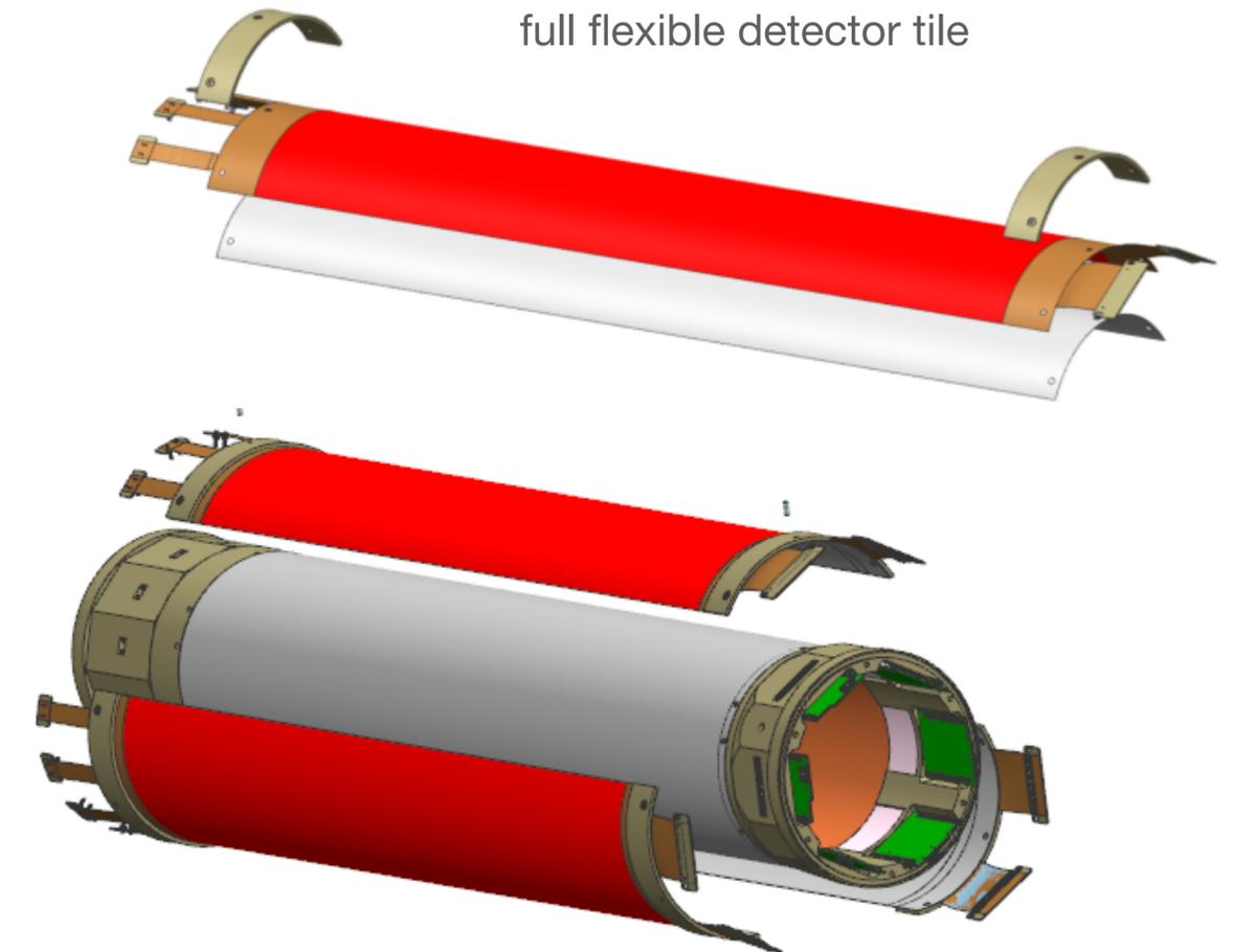
Three of such flexible detector tiles are glued on composite/foam roof-tiles, then mounted on the anode cylindrical support
