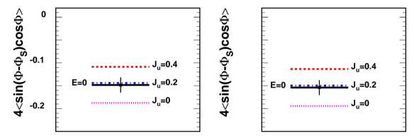
Expected DVCS asymmetry  $A_{UT}^{\sin(\phi-\phi_S)\cos\phi}$  with  $b_v = 1, b_s = \infty, J_u = 0.4(0.2, 0.0), J_d = 0.0$  in the Regge (left panel) and factorized (right panel) ansatz, at the average kinematics of the full measurement. E = 0 denotes zero effective contribution from the GPD E. The projected statistical error for 8M DIS events is shown. The systematic error is expected to not exceed the statistical one.
