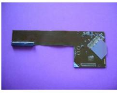
Hybrid board with detector and VFAT front-end chips.
