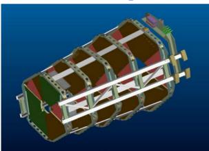
Mechanical frames and CSC detectors in production; tests in progress. Installation depends on CMS.
