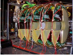
75 % of GEM chambers produced and tested up to a gain of 8 x  $10^4$ .
