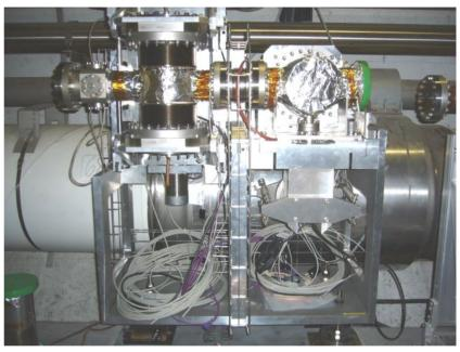
"Edgeless" silicon strip detectors in production; tests in progress.
