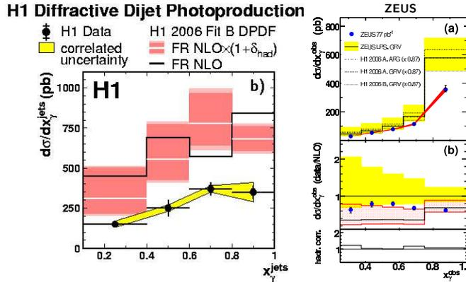
Fig. 1: The differential cross section for diffractive dijet production in  $\gamma p$  scattering as a function of the fraction of the photon momentum involved in the interaction,  $x_{\gamma}^{jets}$  or  $x_{\gamma}^{obs}$ , as measured by H1 (left) and by ZEUS (right).
