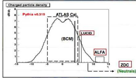
Fig. 4: The  $\eta$  coverage in the ATLAS experiment.
