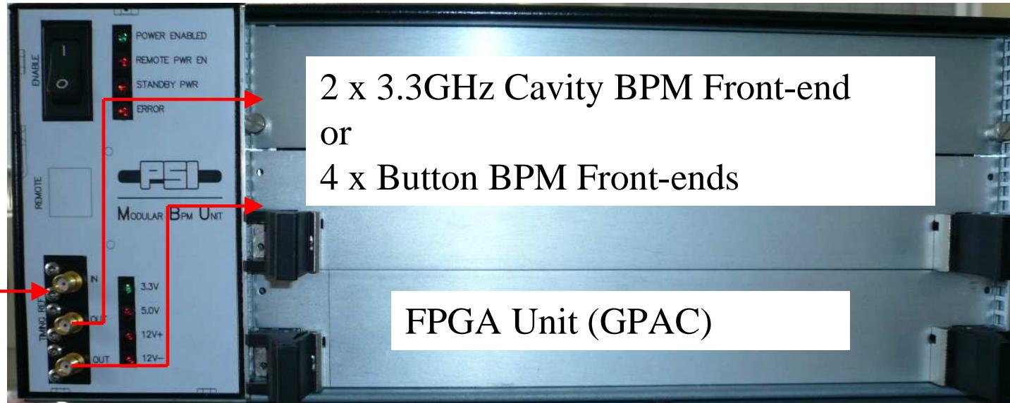
2 x 3.3GHz Cavity BPM Front-end
