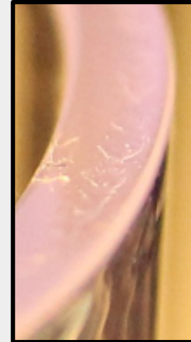
Residue from coating process on one of the surfaces (both tubes)
