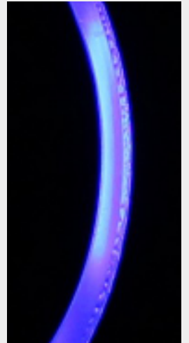
Residue from coating process on one of the surfaces (both tubes)
